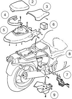
Loosen and remove the rear end cover by removing the six attachment bolts and the six plastic fasteners.
