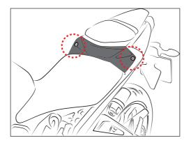
Remove the front seat, by removing the 2 screws.
