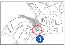
Loosen the bolts (1) (2) the screws (3) (4) (5) (6) and pull the locating pins (7) (8) out of the rubber grommets and remove the tail fearing.
